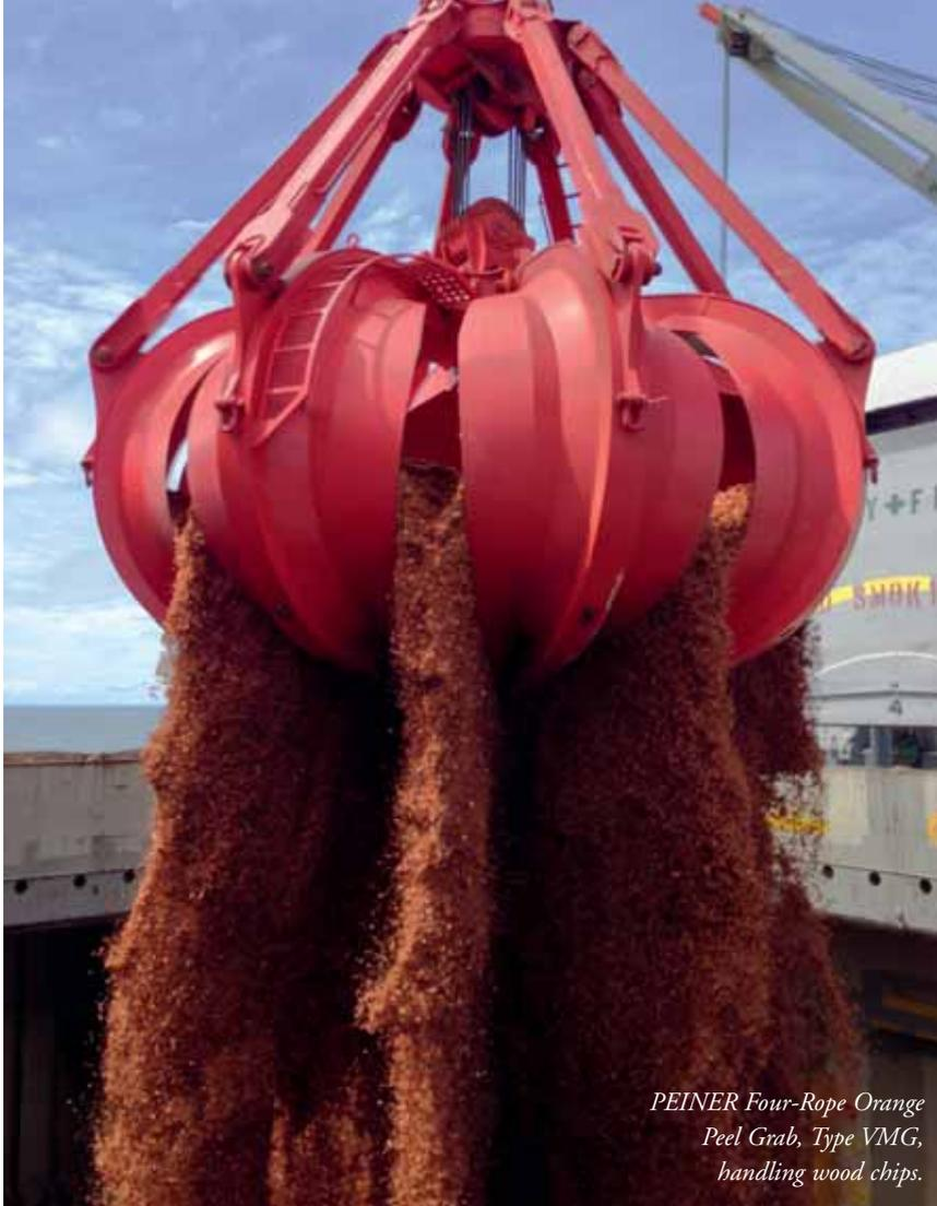
*PEINER Four-Rope Orange Peel Grab, Type VMG, handling wood chips.*
