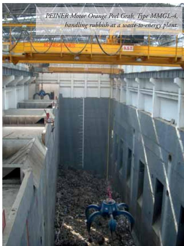
*PEINER Motor Orange Peel Grab, Type MMGL-4, handling rubbish at a waste-to-energy plant.*
